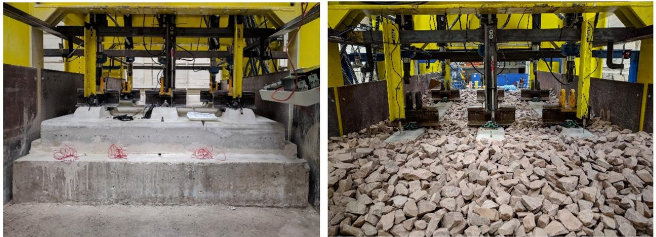
Figure 4. Slab track and ballasted track in GRAFT-2, respectively.
