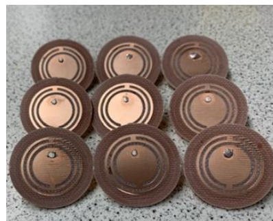
Figure 3. Fabricated antennas using LPKF ProtoMat D104
